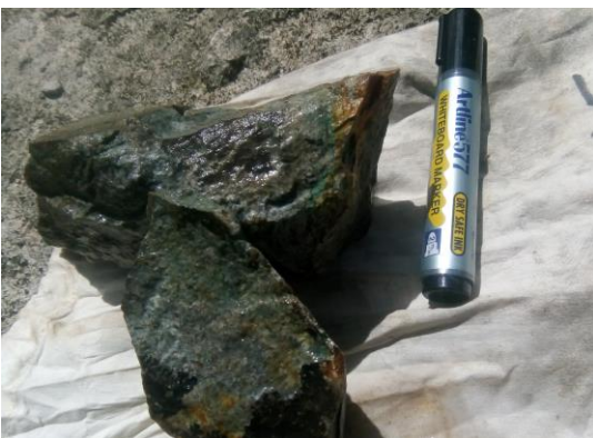
Figure 2: Sample KT515 (malachite bearing intrusive; 2040ppm Cu)
